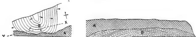
Horizontal and vertical section of small fold on shore 2\frac{1}{2} miles N.W. of Red Island. A, A, trappean rocks. B, B, reddish and greenish shales. X—Y, line of section 200 ft. long.
